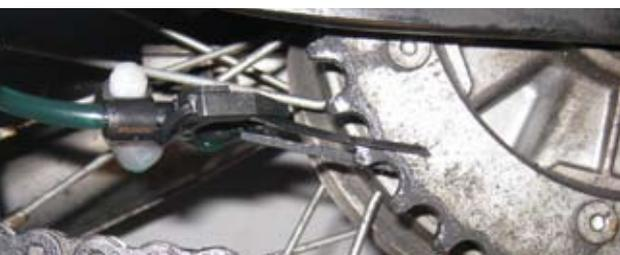
In the first month the bottle came loose and rubbed against the wheel puncturing itself. A replacement bottle is available and will be cable tied in place this time to prevent this happening again.
